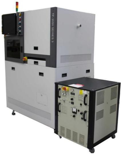
The **TF-3050 Series 3 LDP15TQ** provides high accuracy performance to overcome the new challenges of smaller geometries of chip resistor trimming. Proprietary designs achieve the high accuracy mechanical positioning and ultra-stable laser beam control demanded by industry. **TF-3050 S3** utilizes vision registration theta rotation within a Windows XP operating system. These advance features are integrated with established substrate handling and automation systems.
